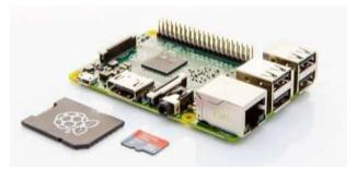
It is a remarkable device link a tiny computer available in lowest package. This s le like a computer which contains CPU, Memory and GPU. It has SOC, RAM, Radio Module, PMIC, USB ports, Pi camera module, HDMI port, DSI, Raspatch touch screen display, GPIO.
