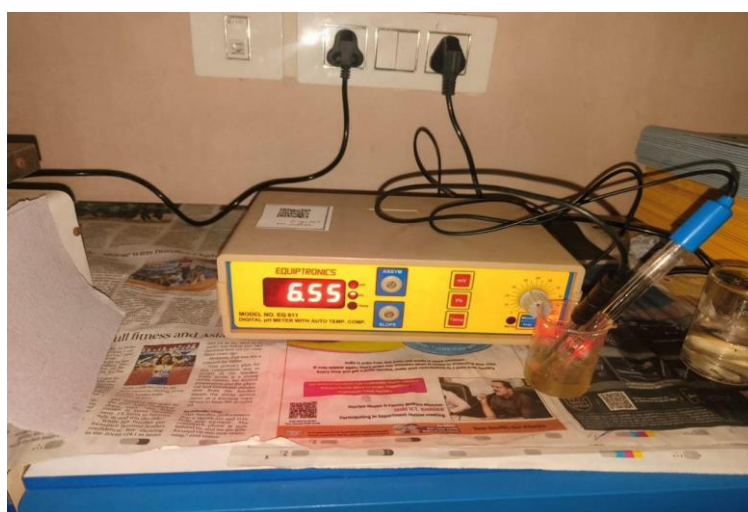
Fig. 4.02: pH Determination of Caffeine extract
