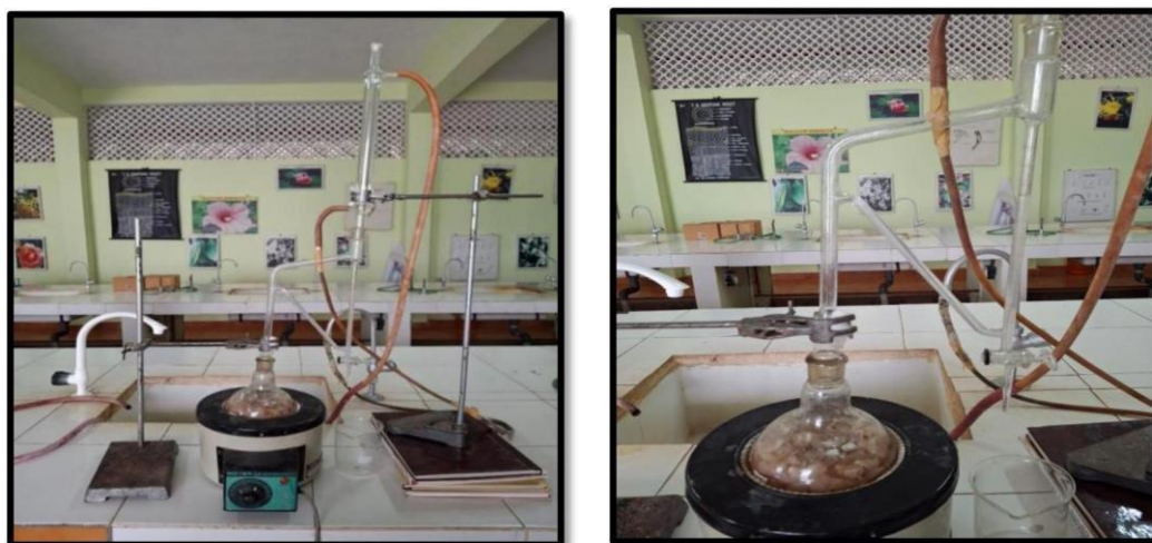
Fig no 2: Extraction of volatile oil of Allium cepa L aggregatum
