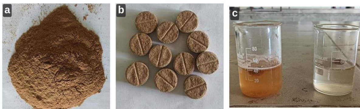
Figure 1. (a) Dried bael fruit extract powder. (b) Compressed floating tablets. (c) Comparative appearance of the dissolution medium during the in vitro buoyancy study, with floating tablets at the surface.
