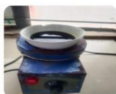
4. plant extracted heated by Heating Mantle to remove ethanol.
