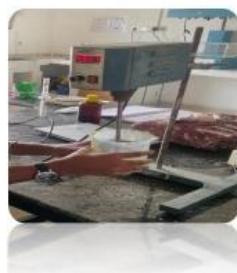
8. Hot aqueous phase is added To lipid phase and homogeneized At high speed.
