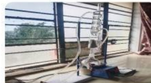
3. Powdered plant material extracted Using ethanol by Soxhlet apparatus.
