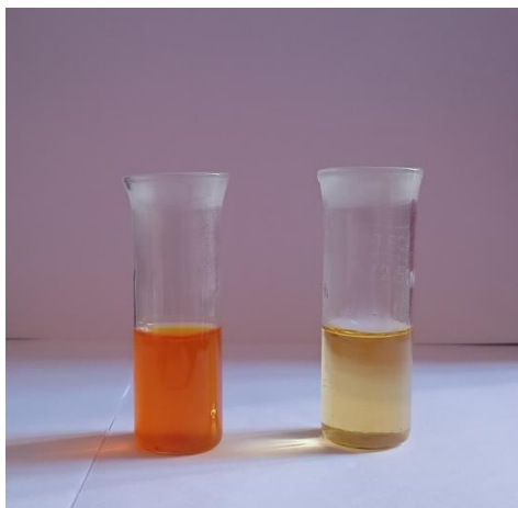
Figure 3C. Comparison of methyl orange solution before and after adsorption.
