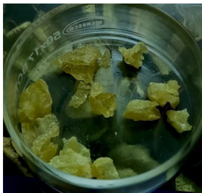
Figure 1. Photograph of the prepared guar gum-g-poly(acrylic acid) superabsorbent composite (SAC 1).
