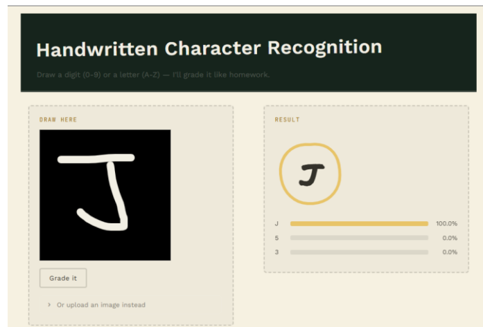
Fig. 2 - Screenshot of the web application showing a drawn character, the predicted character and the top-three confidence scores.
