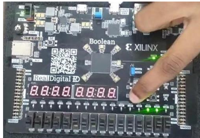
Fig. 10. FPGA output when ALU_Sel is 100 (XOR)
