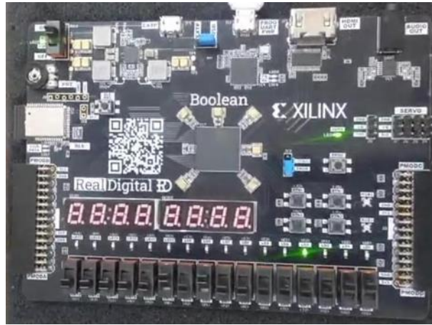
Fig. 2. Boolean board (Spartan-7 XC7S50) used for prototyping the ALU.
