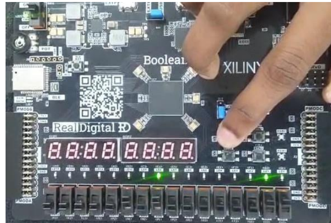
Fig. 7. FPGA output when ALU_Sel is 001 (SUB)
