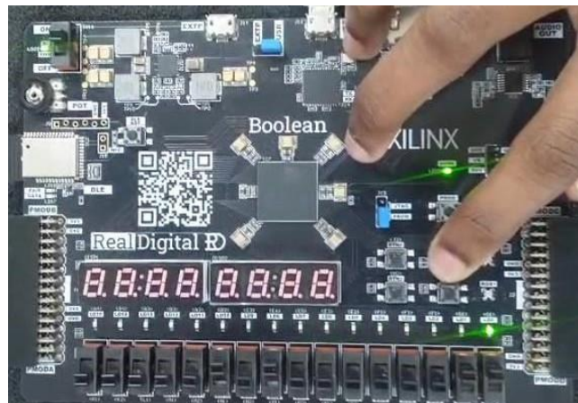
Fig. 8. FPGA output when ALU_Sel is 010 (AND).
