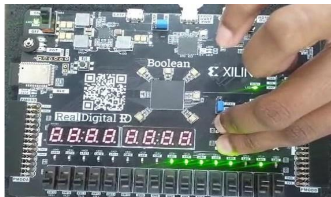
Fig. 11. FPGA output when ALU_Sel is 101 (NOT)
