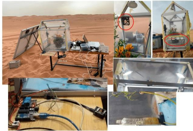
Fig. 5 - Greenhouse farm powered by the PV system in the Sahara (from [4])
