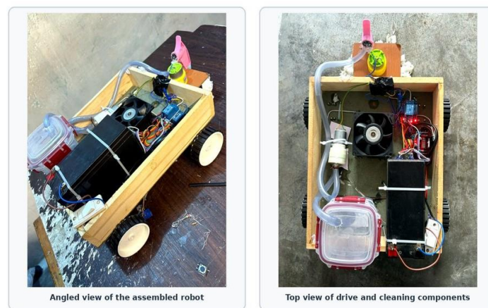
Fig. 3. Photographs of the physical prototype showing the assembled chassis and internal components.
