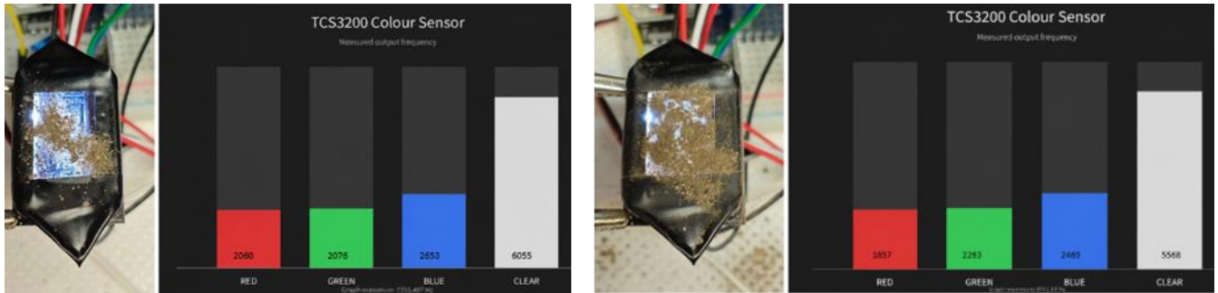
Fig. 4 - Comparison of TCS3200 sensor frequency outputs for RGB channels under mild and heavy soiling levels in indoor conditions.
