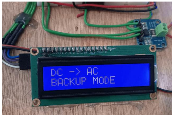
Fig. 4. LCD display photographs: (a) AC→DC mains-available screen; (b) DC→AC backup-mode screen.
