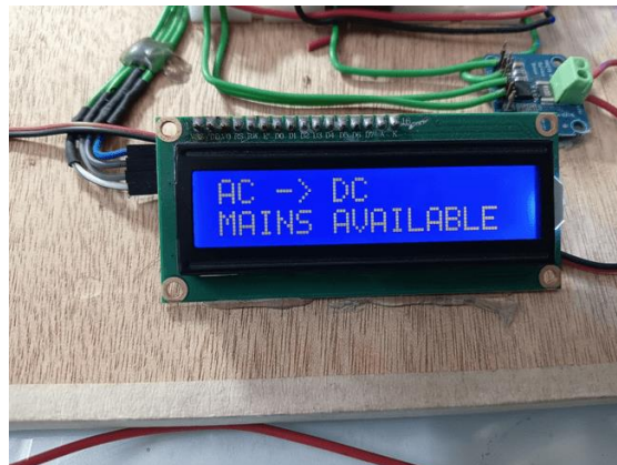
Fig. 4. LCD display photographs: (a) AC→DC mains-available screen; (b) DC→AC backup-mode screen.
