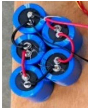
Fig. 3. Series-connected supercapacitor cells on the prototype board.
