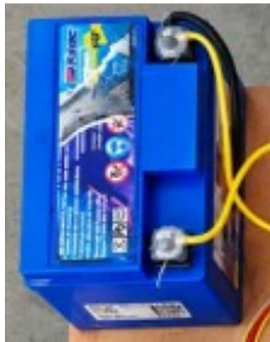
Fig. 2. Lead-acid battery on the prototype board.
