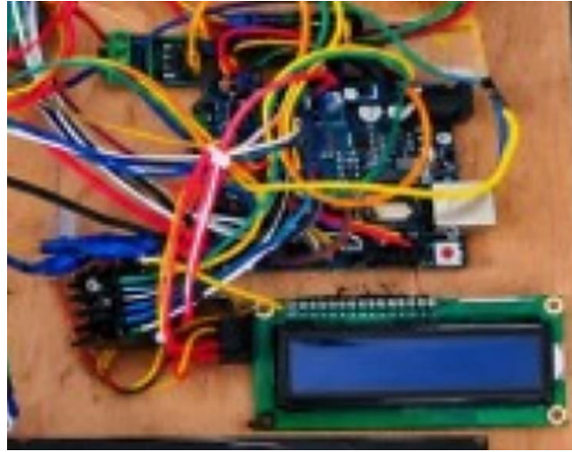
Fig. 9. Arduino board and the 16×2 LCD on the prototype.
