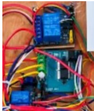
Fig. 16. Relay modules on the prototype board.
