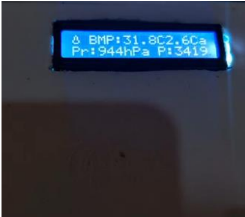
Plate 5: ESP32 Gateway Displaying Local Sensor Readings
