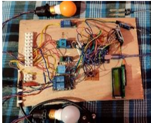
Fig. 1. Prototype of the Proposed Intelligent Earthing Health Monitoring System
