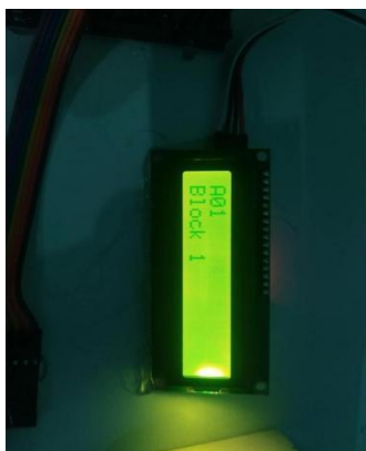
Figure 5: (a) LCD showing book location, (b) LED indication on the correct shelf, (c) buzzer alert on book misplacement
