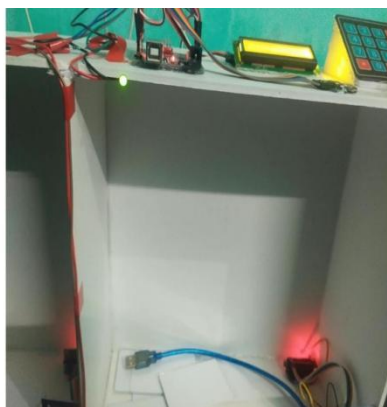
Figure 5: (a) LCD showing book location, (b) LED indication on the correct shelf, (c) buzzer alert on book misplacement
