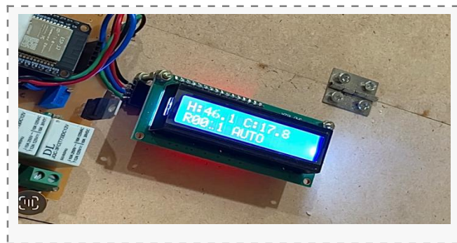
Fig. 6. LCD showing the live hot-side (H) and cold-side (C) temperatures, relay status and AUTO mode during a test run.
