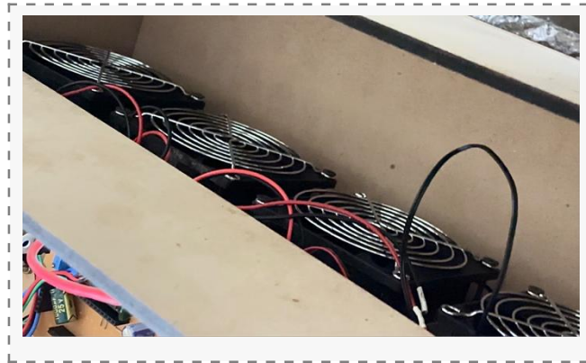
Fig. 4. Interior of the food chamber showing the Peltier modules, heat sinks, fans and temperature sensors.
