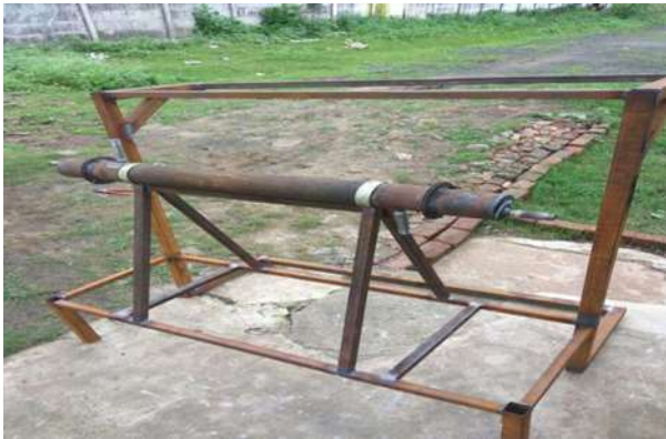
Fig. 4.1: Heat exchanger with flange and tape insertion
