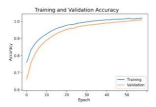
The training accuracy reached **97.45%**, while the validation accuracy stabilized at **96.85%**, indicating good generalization. The training loss decreased consistently, converging near 0.08, confirming effective optimization.
