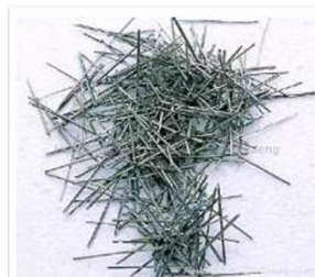
Steel Fibres Extracted from Binding Wire
