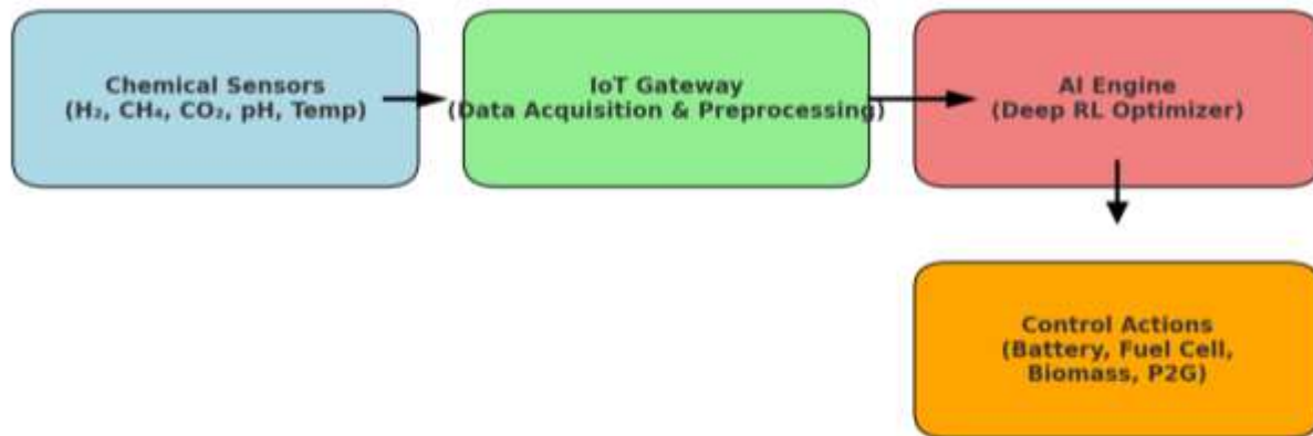
Figure 2: Data Flow from Smart Chemical Sensors to Control Actions
