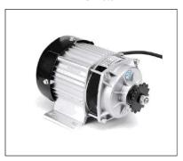
A Brushless DC (BLDC) motor is an electric motor that runs on direct current (DC) power but doesn't have the brushes and commutator that other DC motors do. It uses an electronic controller to switch the current to the motor windings instead of brushes. This creates a magnetic field that moves a rotor with a permanent magnet.
