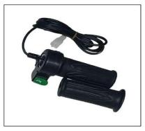
A throttle on an electric vehicle is not a mechanical part; it's an electronic part. It doesn't control the flow of air and fuel in a gasoline engine. Instead, it sends a message to the motor controller, which then decides how much power goes from the battery to the electric motor.
