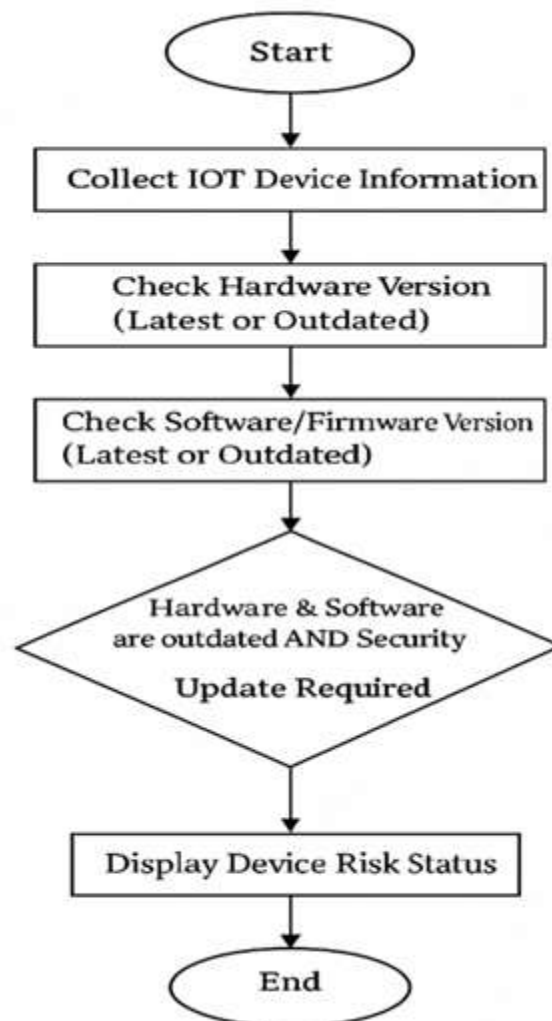
Fig.1.Framework for Identifying and Classifying Vulnerable IoT Devices.
