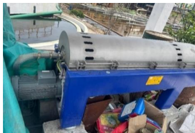
Figure 4.6 Centrifuge machine for Dewatering Sludge
