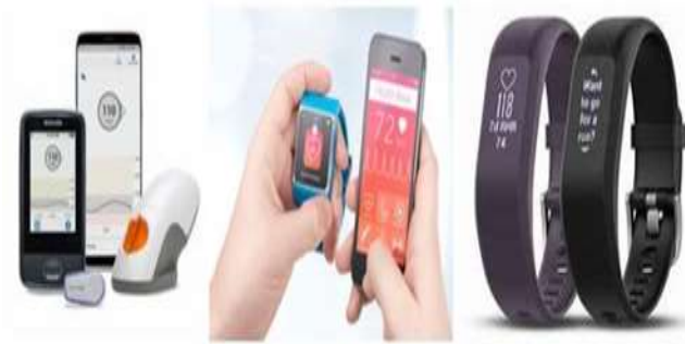
Fig. 3. Wearable devices for health monitoring: (a) Continuous glucose monitor showing glucose trends, (b) Smartwatch displaying heart rate, and (c) Fitness tracker tracking activity.
