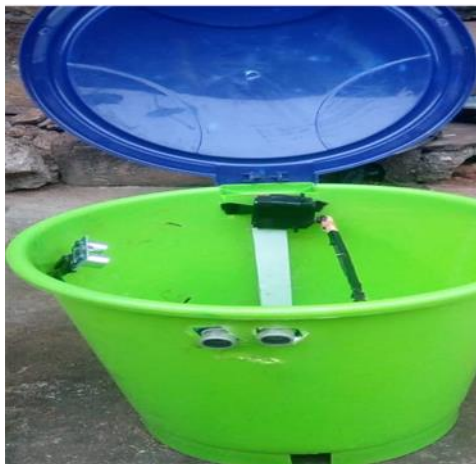
Fig.3.2 Diagram showing how Servo motor was placed on the Trash Bin
