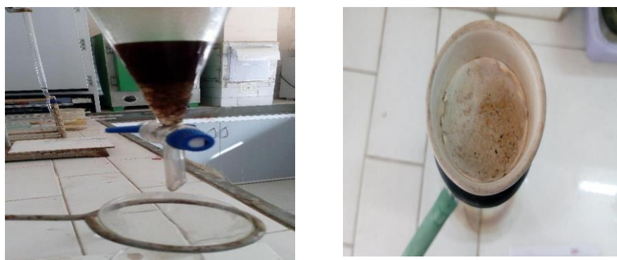
Figure 4: Separation of Glycerol and Methyl Ester
