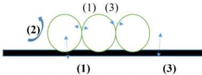
Fig 1: Heat transfer modes within dusty surface-side view including: (1) conduction, (2) convection, and (3) radiation.
