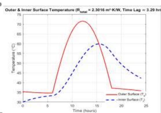
Fig 7 Dust Cool Roof Thermal Performance
