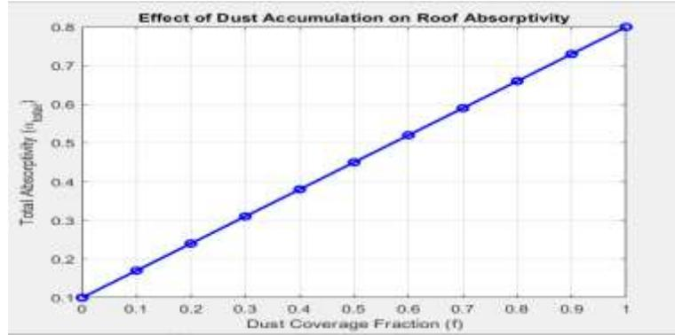
Fig3 Relationship between roof solar absorptivity and dust accumulation
