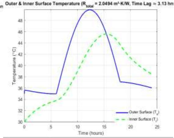
Fig 10 Dust Cool Roof Thermal Performance
