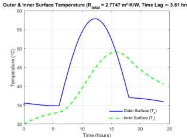
Figure 11 New cool Roof Thermal Performance
