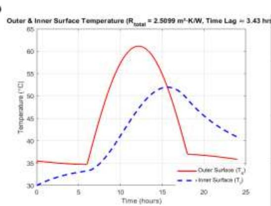
Fig 9 Dust Cool Roof Thermal Performance
