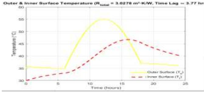
Figure 13 New cool Roof Thermal Performance
