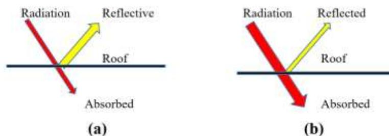
Fig 2: Variation of absorbed solar radiation under two roof conditions; (a) clean roof and (b) dusty roof.
