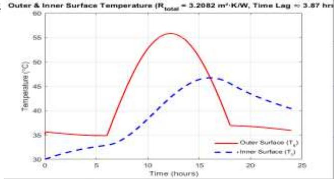
Fig 16 Dust Cool Roof Thermal Performance
