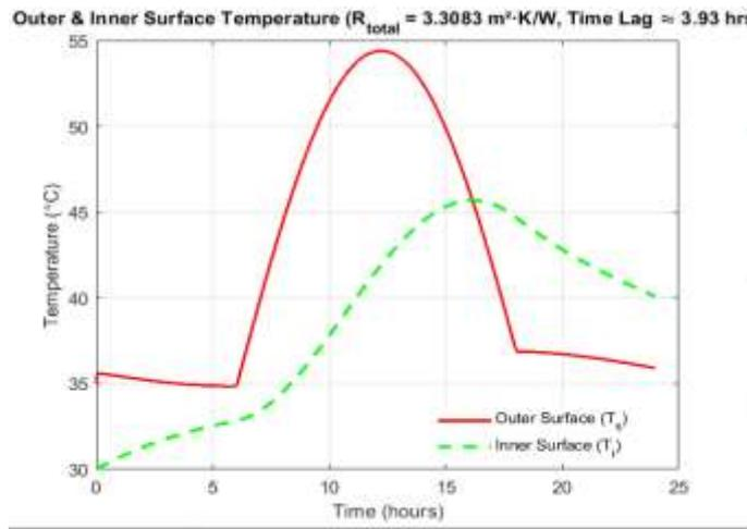
Figure 17 New cool Roof Thermal Performance
