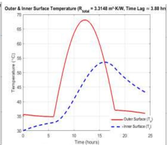
Fig 18 Dust Cool Roof Thermal Performance
