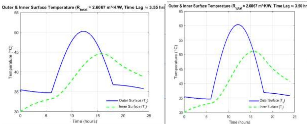
Figure 4 New Cool Roof Thermal Performance
