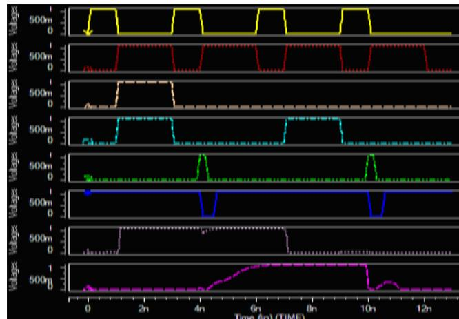
**Figure: 4T1SRAM Wave forms**
