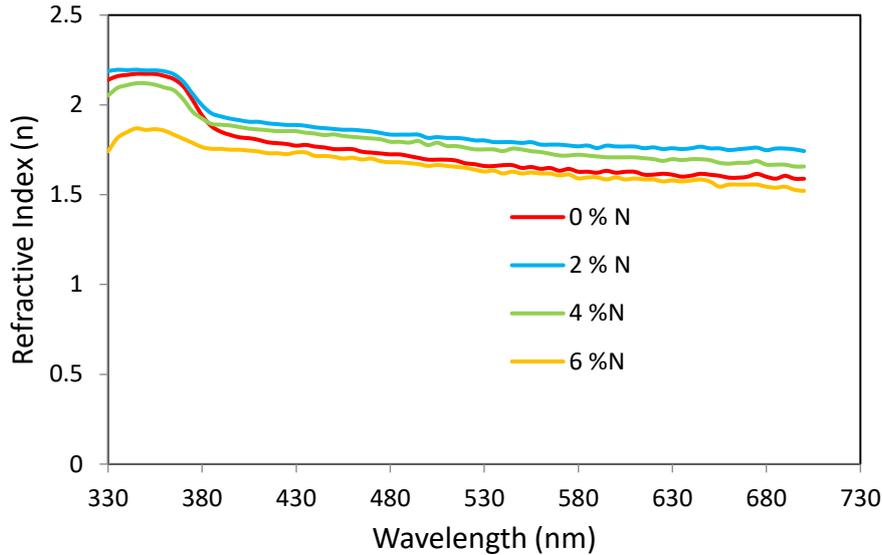
Figure 7: Plot of Refractive Index against Wavelength (nm) for ZnO and N- ZnO Thin Films.
