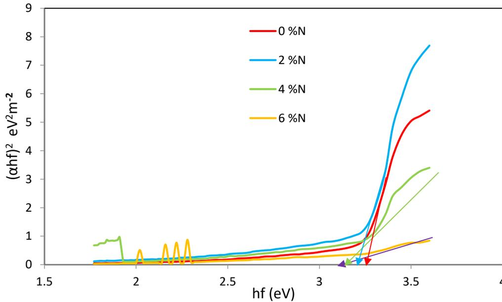
Figure 4. Plot  $(\alpha hf)^2 \text{ eV}^2 \text{ m}^{-2}$  against  $hf \text{ (eV)}$  for ZnO and N- ZnO Thin Films.
