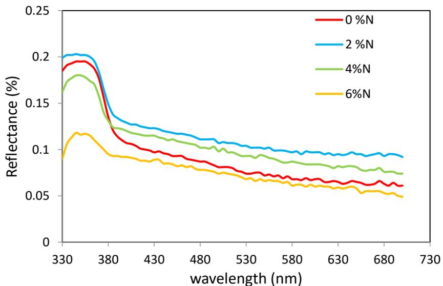
Figure 3: Plot of Reflectance (%) against wavelength (nm) for ZnO and N- ZnO Thin Films.
