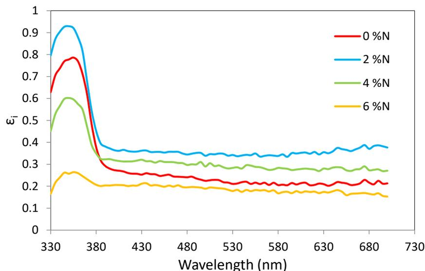
Figure 9: Plot of Imaginary Part of Dielectric Constant against Wavelength (nm) for ZnO and N- ZnO Thin Films.
