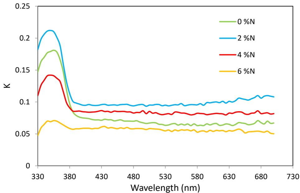
Figure 6: Plot of Extinction Coefficient against Wavelength (nm) for ZnO and N- ZnO thin films.
