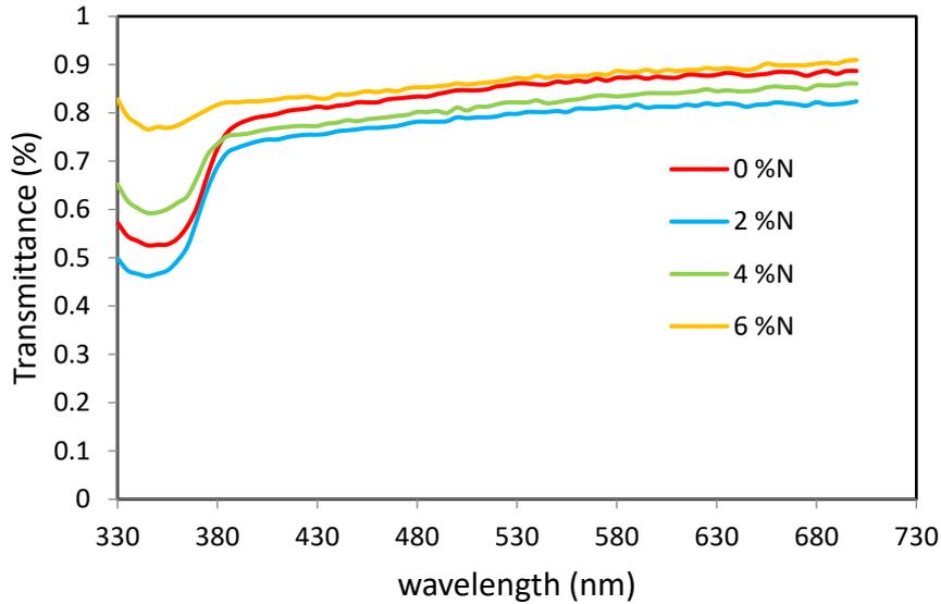
Figure 2: Plot of Transmittance (%) against wavelength (nm) for ZnO and N- ZnO Thin Films.
