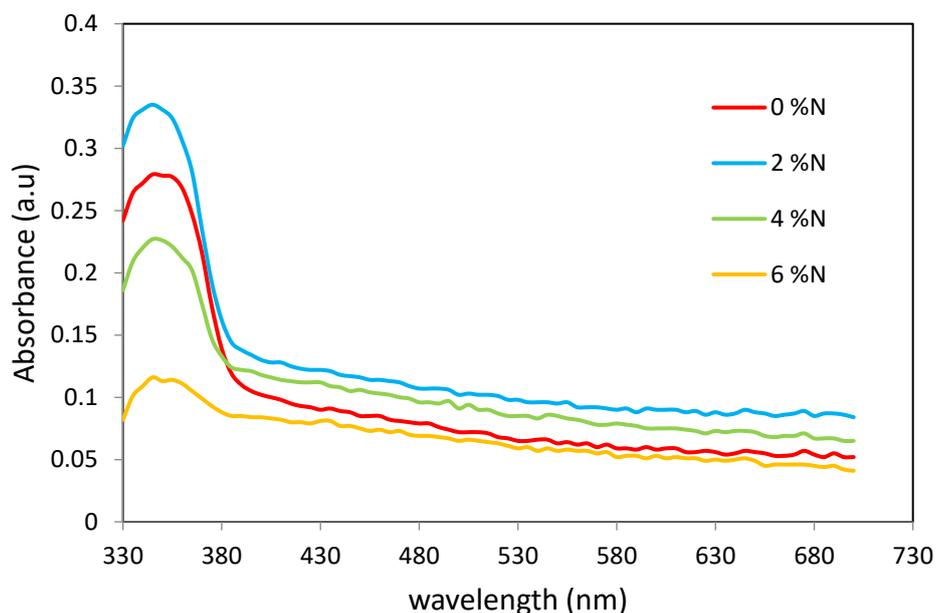
Figure 1. Plot of absorbance against wavelength (nm) for ZnO and N- ZnO Thin Films.
