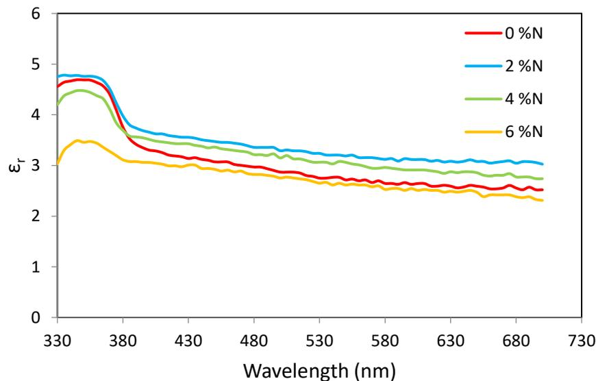
Figure 8: Plot of Real Part of Dielectric Constant against Wavelength (nm) for ZnO and N- ZnO Thin Films.
