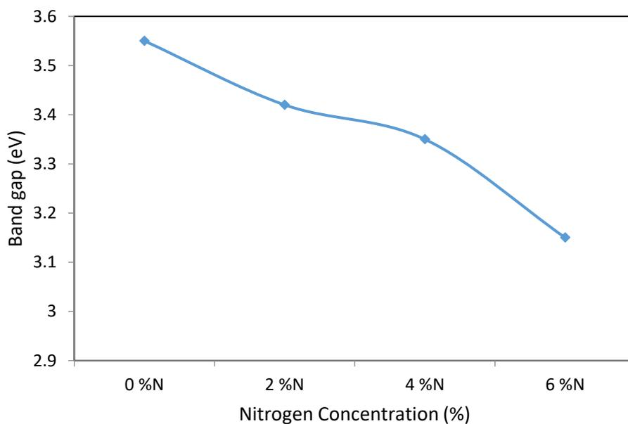
Figure 5: Plot of the Variation of Band gap (eV) with Nitrogen Concentration (%) for ZnO and N- ZnO Thin Films.
