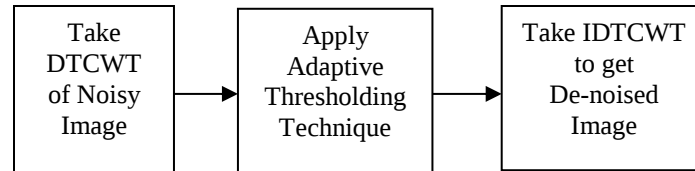
Fig. 1.3 DTCWT based image de-noising method
