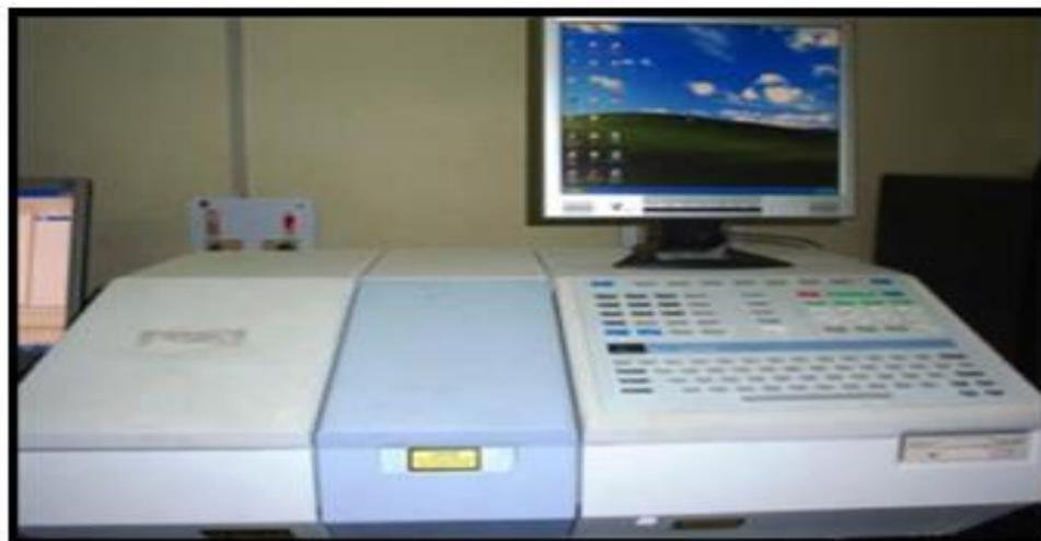
Figure 3: Perkin-elmer spectrum RXI, (FTIR) spectrometer
