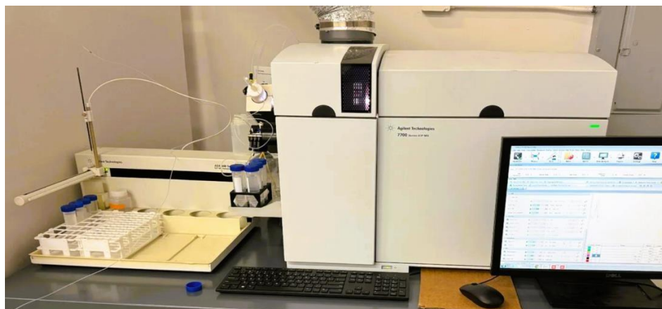
Figure No: 4: Toxic metal contamination using Inductively Coupled Plasma Mass Spectrometry (ICP-MS)
