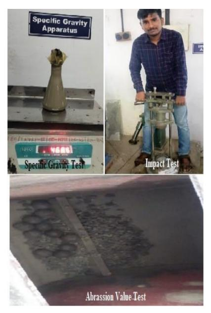
The following tests were conducted in order to determine the properties of modified bitumen.
