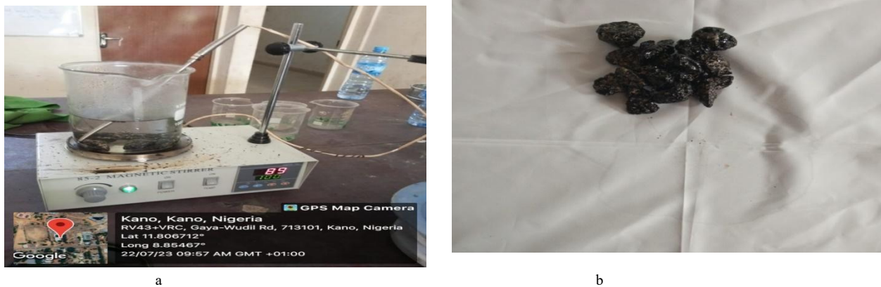
Figure 2.0 Boiling Water Test: (a) Boiling Water Test Assembly and (b) the Prepared loose Mixture
