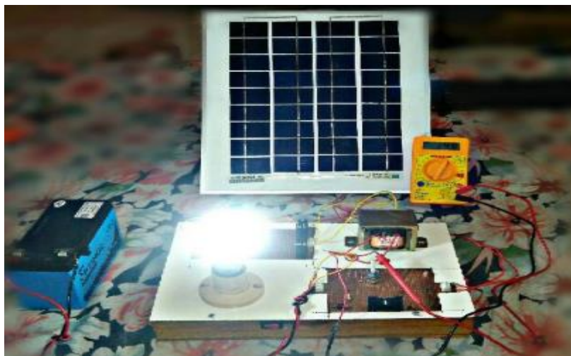
Fig. Solar-Powered Uninterruptible Power Supply
