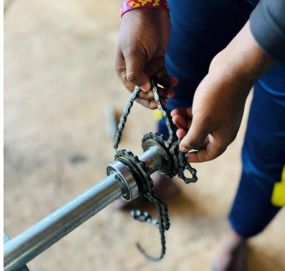
Figure 6: Assembling ratchet mechanism
