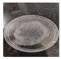
Manual testing of the films revealed moderate flexibility, suggesting that the material could be viable for packaging applications that require pliable yet durable films. The samples also demonstrated reasonable tensile strength, as evidenced by their resistance to tearing under hand-applied pressure.
