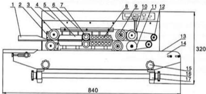
This machine is made up of rack, speed-regulating mechanism, sealing temperature control system, transmission and conveying system etc.
