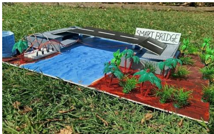
Fig. 5 - An increased water level is detected by the soil moisture sensor
