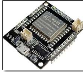
Fig.2 VC-02 Voice recognition Module
