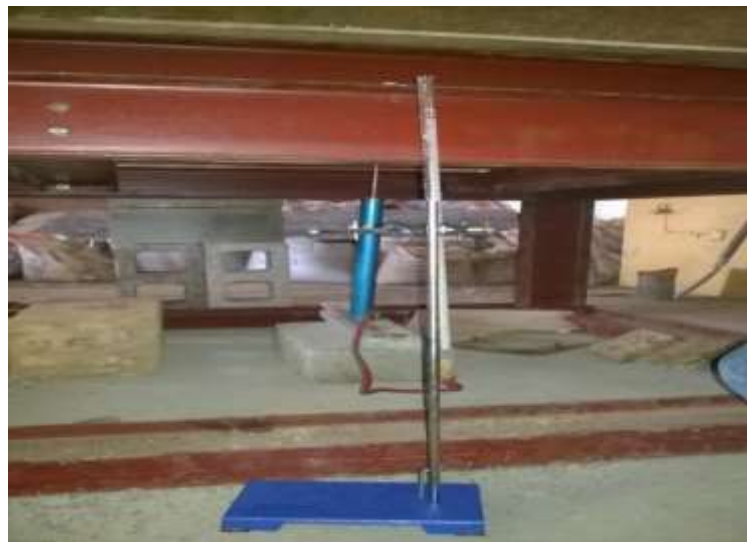
Plate 4.2: Deflection measurement using principle of incompressibility of water
