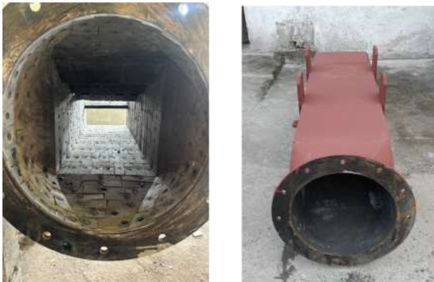
10 mm thick weld-on Ceramic liner fitted inside surface of Coal Burner Transition Piece
