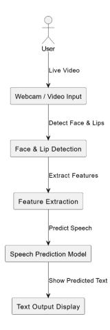
The *Lip Detection and Speech Prediction System* works by analysing live video feed from a camera, detecting facial and lip movements, extracting meaningful features, and predicting the corresponding speech content without requiring any audio input. The entire process is performed in real-time to ensure smooth and responsive communication.
