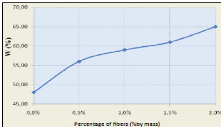
Fig 3: Variation of water absorption of mortar of plaster in function of the percentage by mass of fibers
