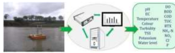
Fig 1: Block diagram of Extraction of IOT Data from Ganga River [1].
