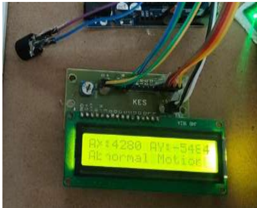
Figure 5: Output during abnormal motion detection
