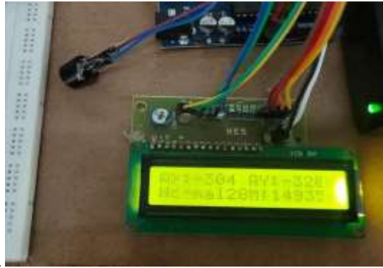
Figure 4: Output during normal motion detection
