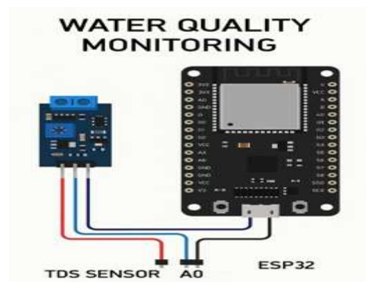
Fig. 4: TDS Sensor Circuit Connection with ESP32
