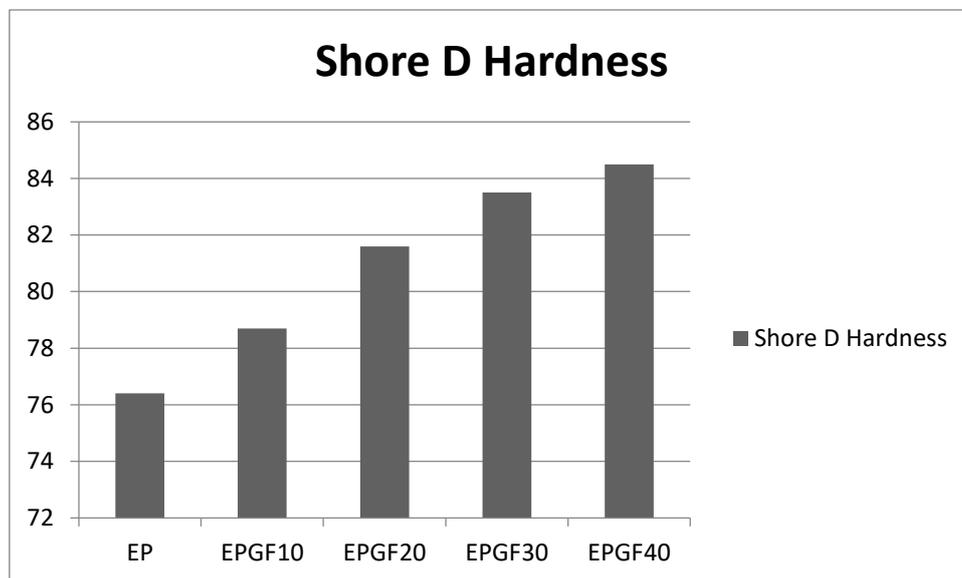
Fig 4 Shore D Hardness of Epoxy-Granite/Fly ash Dust Composites
