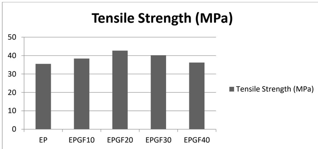
Fig 1 Tensile Strength of Epoxy- Granite Dust fly ash Composites
