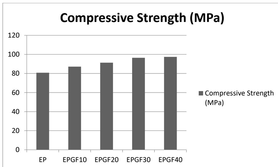
Fig 2 Compressive Strength of Epoxy- Granite Dust/fly ash Composites
