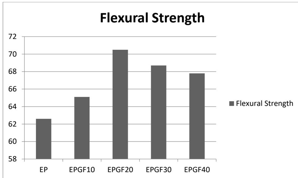
Fig 3 Flexural Strength of Epoxy- Granite Dust/fly ash Composites
