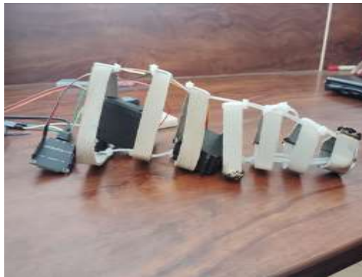
Fig. 3: Prototype of EcoSwim showing fish tail and servo integration.
